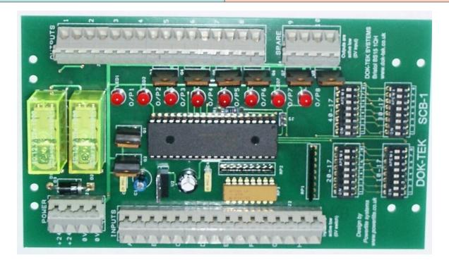
The Software for each mode of operation is contained within the programme PIC controller (The long black rectular item towards the centre of the PCB).
